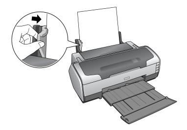
6. Guide the paper into the slot and feed it into the printer until the paper meets resistance.
